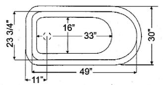
Dimensions of fixture are nominal and may vary within the range of tolerances established by ANSI Standard A112.19.2. Dimensions and specifications subject to change without notice.
